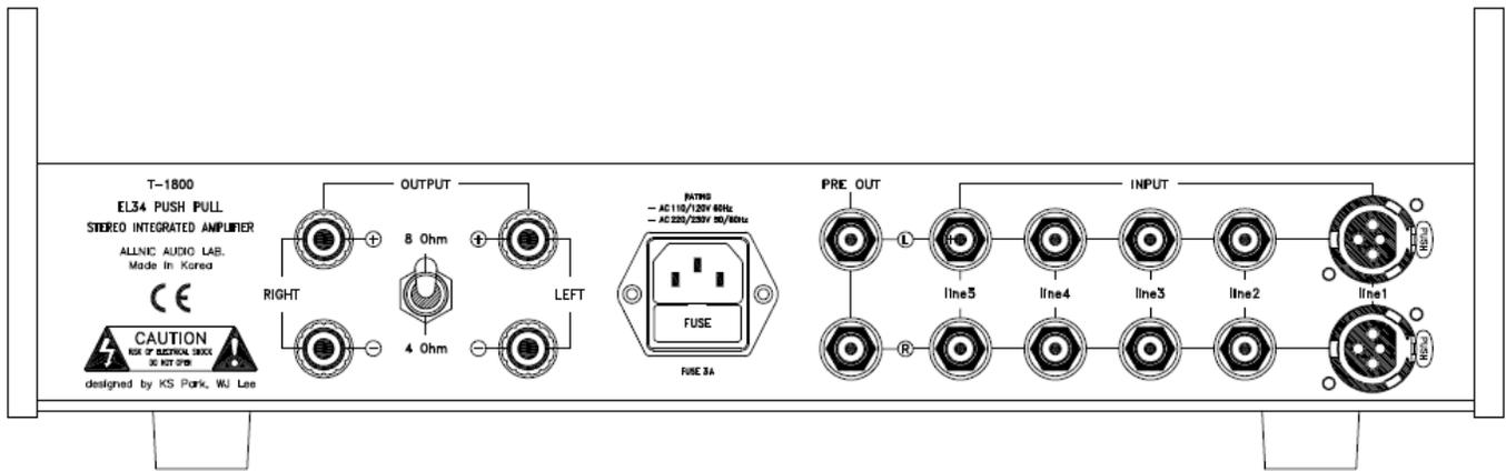
**Figure 3 – T-1800 EL34 Stereo Integrated Amplifier Right-side Panel View**
